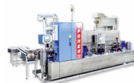
Fig. Continuous cleaning system cleaning/ rinsing/drying with cross conveyor belt and buffer turntable
