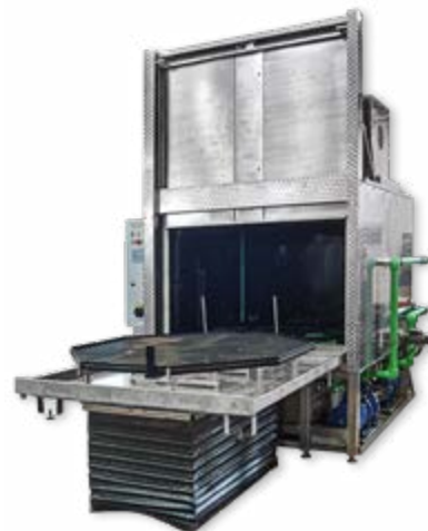
Coated frontloader for cleaning drums with aggressive media
