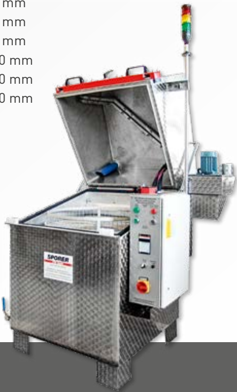
Fig. TRL750 with signal lamp and exhaustion
