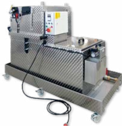
Fig. Modified top loader system for cleaning wire rope ends
